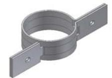
**C-Clamp Assembly** - The c-clamp assembly consists of a c-clamp and clamp bar. The c-clamp assembly is used at each line post to attach the mesh. The c-clamp will fit to the line post on the inside of the fence line while the clamp bar fits to the attack side and holds two pieces of mesh together where they overlap. (ex. CCLAMP3 and CLAMPBAR)
