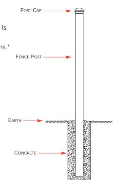
\* Under normal conditions the footer dimension should be 4 times the largest cross section of the post.
