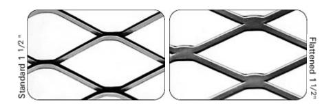
Flattened expanded metal (abbreviated F) is manufactured by passing the metal through a cold roll reducing mill parallel to the LWD. By flattening the sheet, the bonds and strands are turned down to produce a smooth and flat surface – essentially elongating the LWD of the diamond
